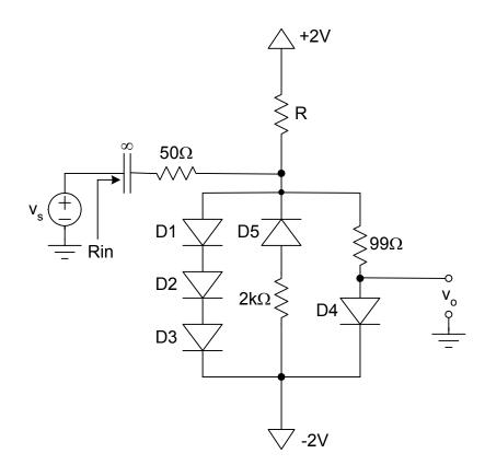
a) [3 pts] Calculate R such that the DC output voltage,  $V_0$ , is -1.25V. Do NOT assume the Constant Voltage Drop model. Hint: all diodes but one are on.
