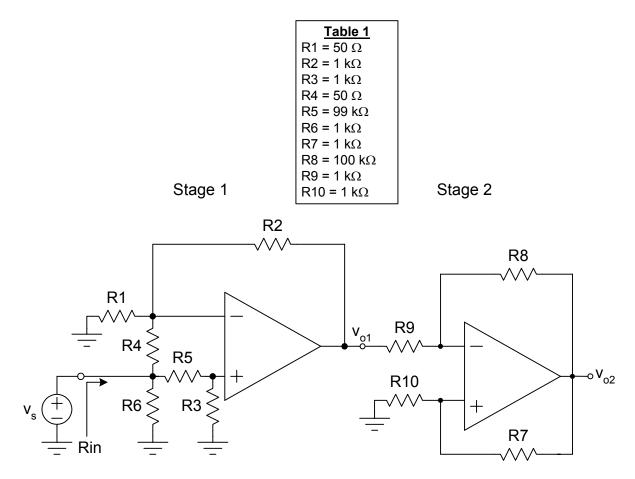
a) [3 pts] Calculate the voltage gain  $(v_{o1}/v_s)$  of the first stage using the resistor values of Table 1.
