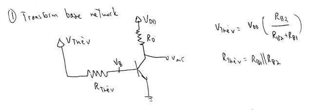
$$V_{D} = V_{DD} - I_{C}, R_{D}$$
