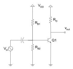
Consider this common-emitter amplifier. You must bias the BJT so that you can get the maximally symmetric output swing. Design assuming a  $V_B$  of 0.7V. Find an expression that relates the resistances  $R_{B2}$ ,  $R_{B1}$  and  $R_D$  to the values of  $V_{DD}$  and  $\beta$ . For  $V_{DD}$ =10V and  $\beta$ =100, choose  $R_{B1}$ =9k $\Omega$ ,  $R_{B2}$ =1k $\Omega$  and calculate  $R_D$ .
