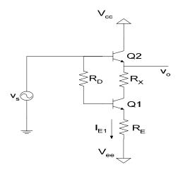
Assume the following:  $v_s = 0$ ,  $R_X = 50\Omega$ ,  $R_D = 70k\Omega$  and  $I_{E1} = 1mA$ . Find a condition on  $\beta$  that ensures that Q1 will be in the active mode. (4 pts)
