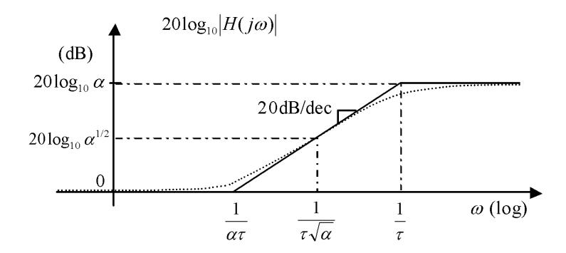
Compare with the first-order lag system, in which  $\alpha < 1$ , the magnitude decrease from a level to a lower level for a system.
