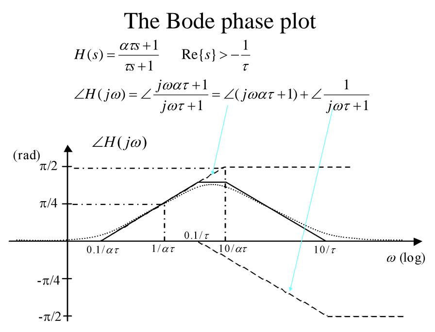
For the case where  $\tau \rightarrow 0$ ,  $\alpha \tau \rightarrow T$ , then the first-order lead is equivalent to a differentiator with gain T in parallel with the identity system: H(s) = Ts + 1
