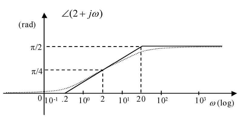
Given a single-zero system (s+2), i.e., the inverse of 1/(s+2), the Bode phase plot is simply the Bode phase plot of 1(s+2) flipped around the frequency axis, because:
