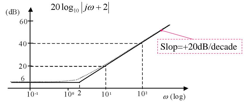
Given a numerator  $(j\omega+2)$ , i.e., the inverse of  $1/(j\omega+2)$ , the Bode magnitude plot is simply the Bode magnitude plot of  $1/(j\omega+2)$  flipped around the frequency axis, because:
