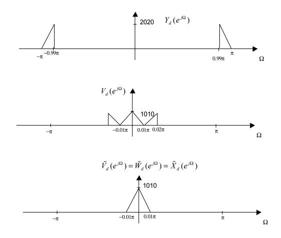
(c) [10 marks] Using the same parameters as in (b), except for  $N_1 = 4$ ,  $N_2 = 2$ , sketch the spectra  $W_d(e^{j\Omega})$ ,  $\tilde{X}_d(e^{j\Omega})$  and  $\tilde{X}(j\omega)$ .
