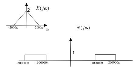
(a) [6 marks] Find the minimum antialiasing filter's cutoff frequency  $\omega_a$  that will avoid any unrepairable distortion of the modulated signals due to the additive noise n(t). Sketch the spectra  $Y_n(j\omega)$  and  $W(j\omega)$  of signals  $y_n(t)$  and w(t) for the frequency  $\omega_a$  that you found. Indicate the important frequencies and magnitudes on your sketch.
