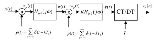
The spectrum  $X(j\omega)$  of the input signal x(t), and the frequency responses of the two ideal lowpass filters, are shown below. The gain of the second lowpass filter is K > 0.
