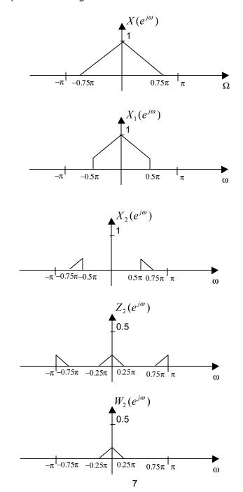
(b) [6 marks] Find the maximum decimation factors  $N_1$  and  $N_2$  avoiding aliasing and sketch the corresponding spectra  $V_1(e^{j\omega})$ ,  $V_2(e^{j\omega})$ , indicating the important frequencies and magnitudes.
