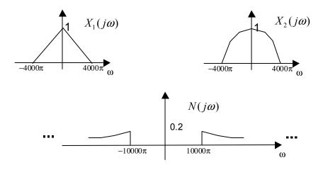
(a) [5 marks] Find the maximum carrier frequency  $\omega_c$  and the corresponding minimum antialiasing filter's cutoff frequency  $\omega_a$  that will avoid any unrepairable distortion of the modulated signals due to the additive noise n(t). Sketch the spectrum  $W(j\omega)$  of the signal w(t) for the frequencies  $\omega_c$  and  $\omega_a$  that you found. Indicate the important frequencies and magnitudes on your sketch.
