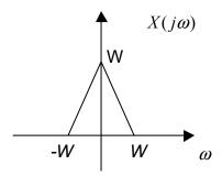
The sampling theorem is satisfied for  $\omega_{s} > 2W$  for the sampler.
