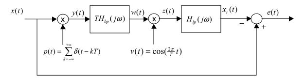
The input signal is  $x(t) = \frac{W^2}{2\pi} \mathrm{sinc}^2 \left(\frac{W}{2\pi}t\right)$  and the spectra of the ideal bandpass filter and the ideal lowpass filters are shown below.
