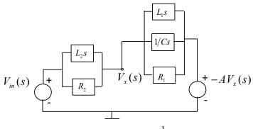
There are two supernodes for which the nodal voltages are given by the source voltages. The remaining nodal equation is
