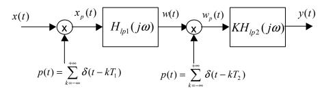
The spectrum  $X(j\omega)$  of the input signal x(t), and the frequency responses of the two ideal lowpass filters, are shown below. The gain of the second lowpass filter is K > 0.
