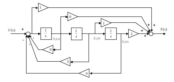
Figure 10.1: Controllable canonical realization of system of Problem 10.2.
