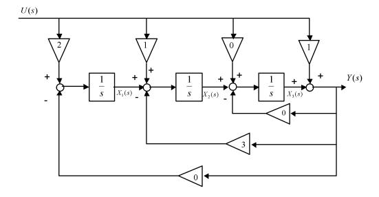
Figure 10.2: Observable canonical realization of system of Problem 10.2.
